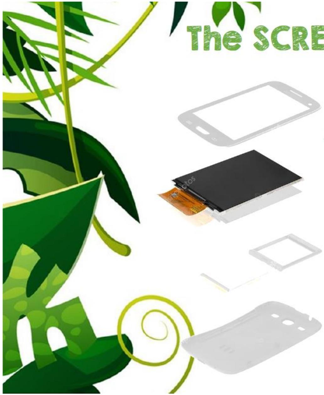
**INDIUM TIN OXIDE** is used in a transparent film that conducts electricity, allowing the screen to function as touch screen.
